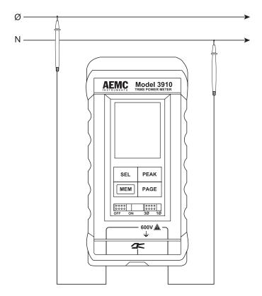
**Note:** The Model 3910 may also measure DC volts. DC will be displayed on the LCD.
