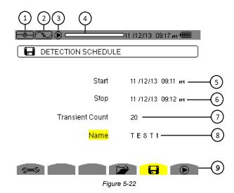
Function Item 1 Reminder of the mode used 2 Display of sub-mode used Flashing Dicon: indicates that the search has been started Memory indicator. Black area = used memory; White area = available memory 4 5 Transients search start time 6 Transients search end time 7 Number of transients 8 Name of transient 9 Display a list of searches; Program a search; Start a search
