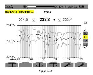
For each of the phases (L1, L2, and L3), at each recording of a value over one second (recording period), the instrument also records the minimum half-cycle RMS value over one second and the maximum half-cycle RMS value over one second. These are the three graphs shown in Figure 5-60.
