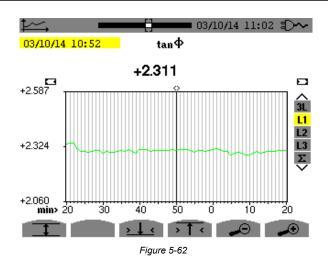
This graph is an example of tan  $\Phi$  (L1) without MIN-AVG-MAX for a 3-phase connection with neutral.
