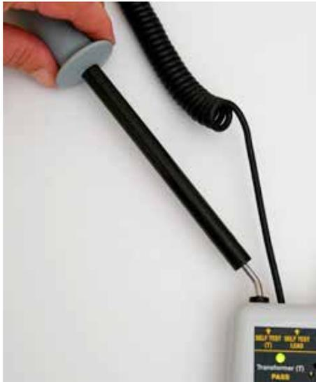
7. Insert the probe into the terminal labeled SELF TEST (C), and press TEST. The green Capacitor (C) PASS light should blink, and the buzzer should sound.
