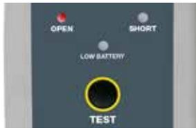
5. Connect the alligator clip to the probe tip, and press the TEST button again. The red SHORT light should blink while you hold down the button.
