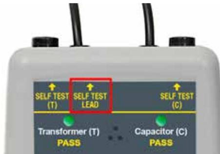
2. Attach the probe to the SELF TEST LEAD by inserting the lead into the probe. Screw the probe into the cable.
