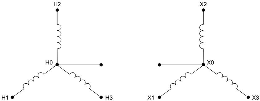
For Y configurations, you must measure from each phase to neutral and from each phase to other phases.
