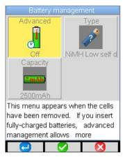
After the batteries are installed (or replaced) the Battery management menu appears when the camera first starts up. This menu can also be displayed by pressing and holding down the **F2** button when the camera is powered ON.
