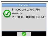
When the file has been saved to the micro SD card, a message displays the name of the file that has just been created (see left for example).
