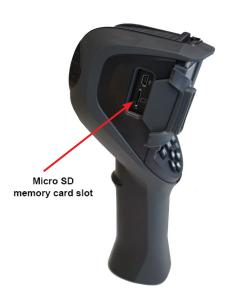
Camera files (images, audio, and setup) are stored in the micro SD memory card located on the left side of the head (see photo to left). If this card is not installed, an error message appears when the camera attempts to access it. This card is provided with the camera.
