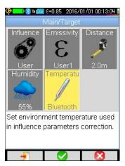
The measurements replace the user data entered in the Target menu (shown left), provided that the Influence setting is User (see § 4.2.2).
