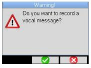
You can create a vocal message for the image. This requires a Bluetooth headset connected to the camera (§ 7.2.1). The recording can be up to 30 seconds long. The vocal message can be added only after you have created the image file. After the message appears displaying the name of the new file, if the headset is connected another message prompts you to record a vocal message (as shown left).
