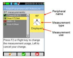
This menu displays measurements received from the connected devices during the last acquisition.
