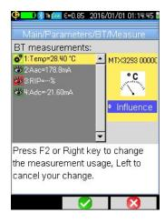
You can use a measurement from a connected device as an **influence** to compensate for an environmental factor. The measurement will be used to calculate the amount of correction that needs to be applied. Note that this option is available only for temperature, humidity, and distance measurements
