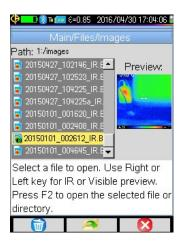
To recall a stored image, ensure the micro SD card is installed in the camera. Then do the following:
