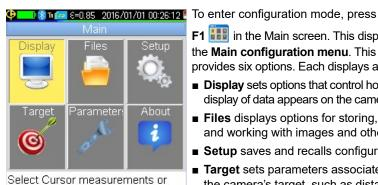
F1 in the Main screen. This displays the Main configuration menu. This screen provides six options. Each displays a submenu:
