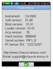
To view the current version of the camera's firmware, select **About** from the Main configuration menu. This displays information about the camera (see example on left). The version number appears on the **Soft version**: line
