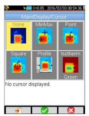
Below the image is the Measurements display area (see § 2.3.1.3). The displayed data depends on the measurement cursor setting. By default, no measurement cursor is selected, resulting in no measurement data displayed in the screen. To change the cursor setting:
