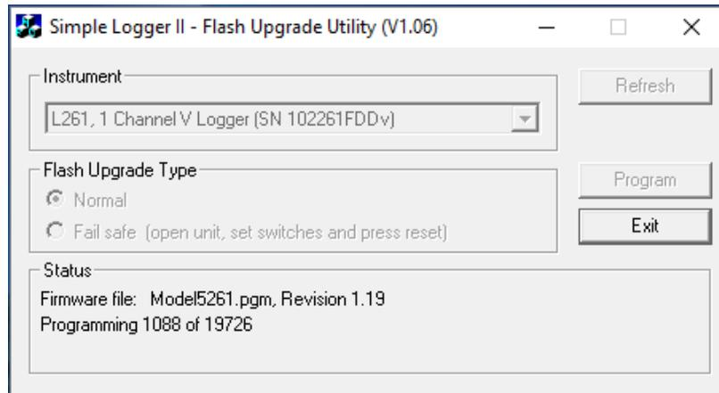
**Step 9:** Once completed the following message will appear. Switch all of the DIP switches to the off position and press reset. (Only applies if Fail Safe upgrade type was used)
