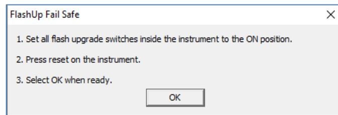
**Step 6:** Locate the flash upgrade switches and reset switch as shown below. Set all switches to the “ON” position and press reset.
